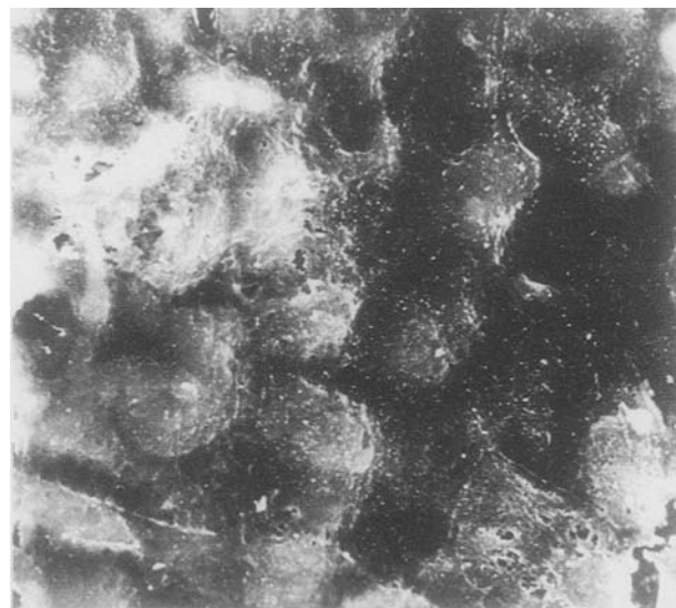
Figure 7 Scanning electron microscopy image of the prosthesis in Fig. 6 showing the dense hydroxyapatite globules of which it consists. They can be seen to be covered by a fine fibrous interface.
