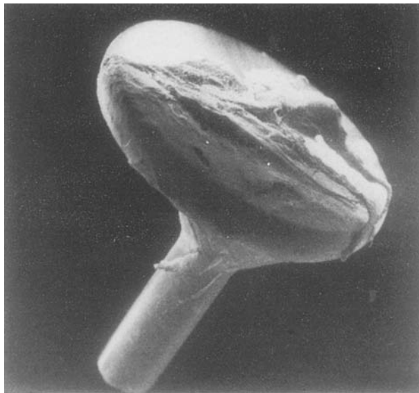
Figure 6 Scanning electron microscopy overview of a hydroxyapatite total ossicular replacement (TORP) removed two years after implantation showing a fine mucosal coating over the platform and the upper part of the stem ( \times 19 ).
